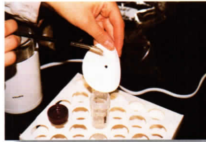
7. Brushing magnetic material into test tube with given volume of solvent to dissolve dye from very fine iron particles.
