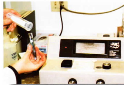
9. Reading color of solution on spectrophotometer.
