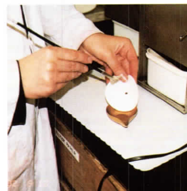
6. Brushing the magnetically retrieved material into a small aluminum weigh scoop, prior to determining particle counts or colorimetric readings.
