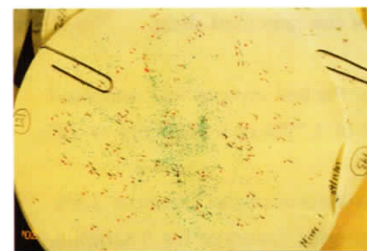
12. Dried 18.5cm filter paper with red particle spots and background fine blue but uncountable color from the very fine colored particles.
