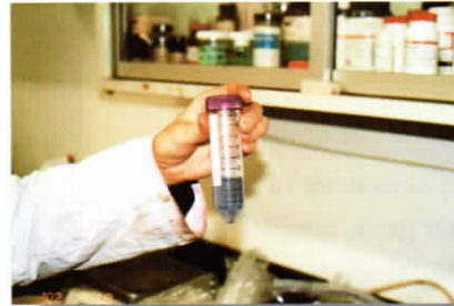
8. Shaking test tube to dissolve dye from tracer particles.
