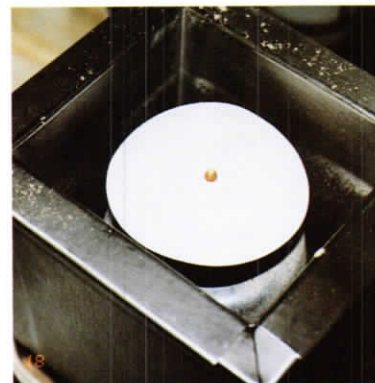
5. Viewing on the 7.5cm filter paper within the Rotary Detector the magnetic materials removed from the feed subsample.
