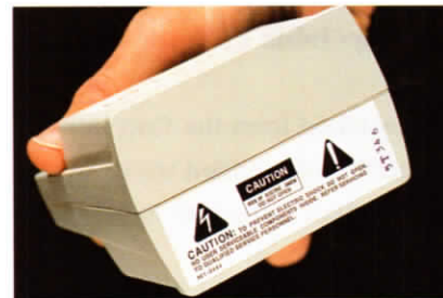
10. "Demagnetizing" the magnetic materials with bulk tape eraser so they do not stick together after magnetic separation from the feed (required for determining particle counts).
