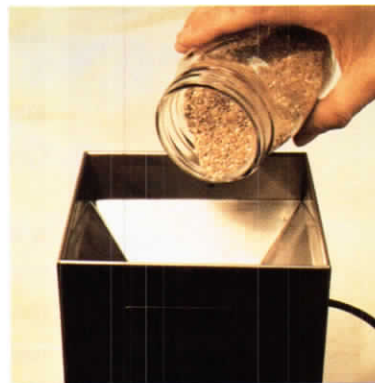
4. Pouring the feed subsample through the upper hopper of the Rotary Detector.
