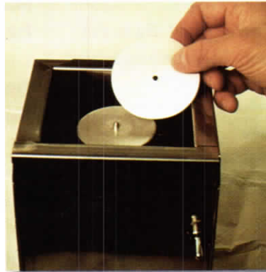
3. Placing a 7.5cm filter paper with centerhole on the circular magnetic platform within the Rotary Detector housing.
