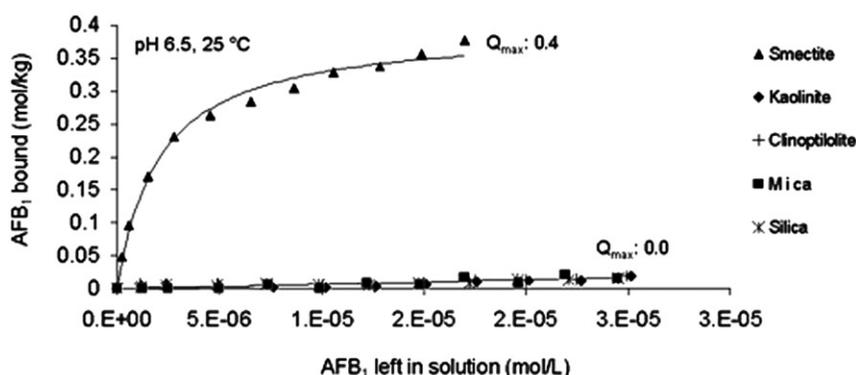
Figure 3. AFB<sub>1</sub> sorption at pH 6.5 on smectite clay (NSP) versus non-binding materials such as kaolinite, clinoptilolite, mica and silica. The highest capacity ( $Q_{max}$ ) for AFB<sub>1</sub> sorption was obtained for smectite (0.4 mol AFB<sub>1</sub>/kg sorbent).  $Q_{max}$  values of 0.0 obtained for the other minerals demonstrate their negligible sorption capacity for AFB<sub>1</sub>. Sorption assays were performed at 25°C.
