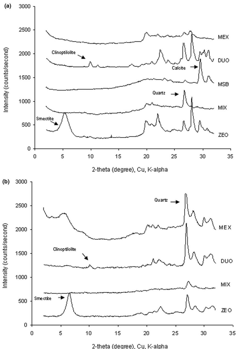
Figure 1. (a) Powder mounts X-ray diffractograms of a smectite containing additive (ZEO) and 4 potential additives without smectite (DUO, MIX, MEX and MSB). (b) Mg<sup>2+</sup> saturated clay samples confirmed the smectite containing additive (ZEO) and the 3 potential samples without smectite (DUO, MIX, MEX). MSB was not included in Figure (b) due to difficulties preparing an oriented sample because of its mainly organic composition. Arrows display the mineral identification of the peaks.
