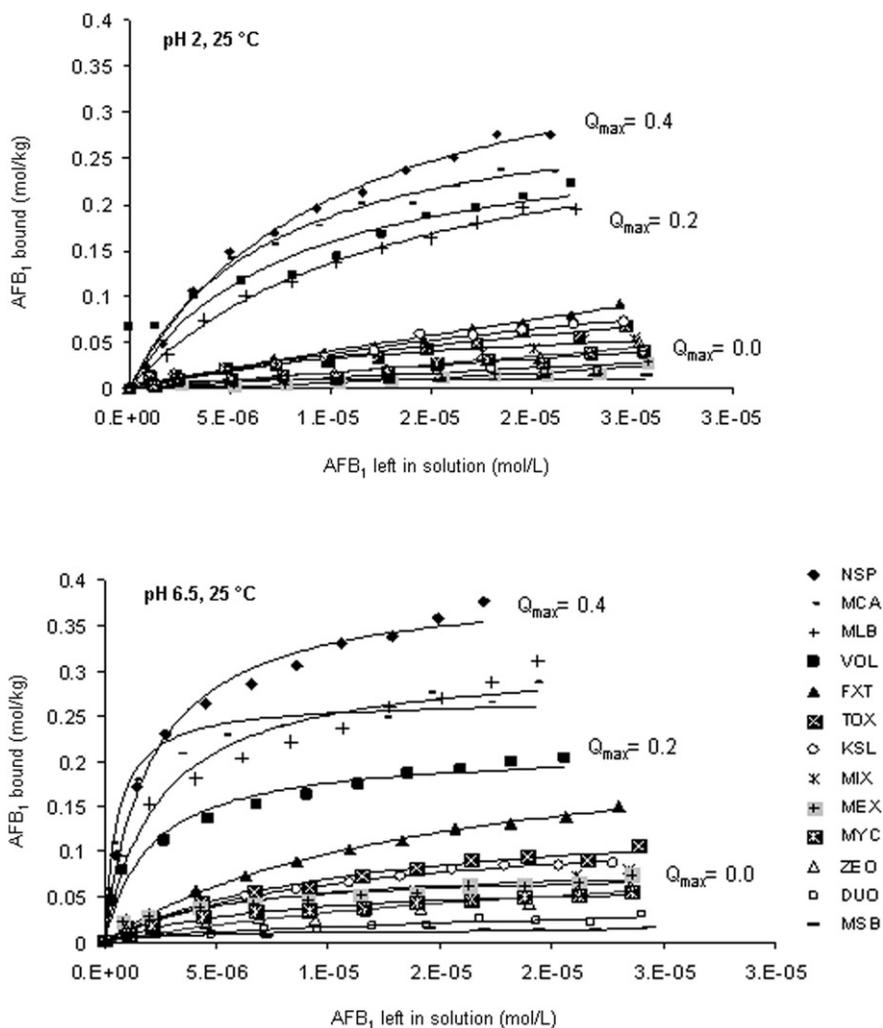
Figure 2. AFB<sub>1</sub> sorption isotherms on binding additives at pH 2 and pH 6.5. Each point represents the values calculated for AFB<sub>1</sub> bound and left in solution for the corresponding 11 dilutions. Isotherms were performed at 25°C.  $Q_{\max}$  is expressed as mol AFB<sub>1</sub>/kg of additive.
